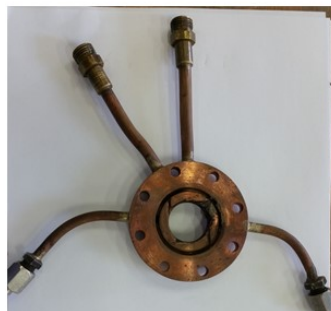
375 GAS INJECTION SEGMENT 1.00 BORE
